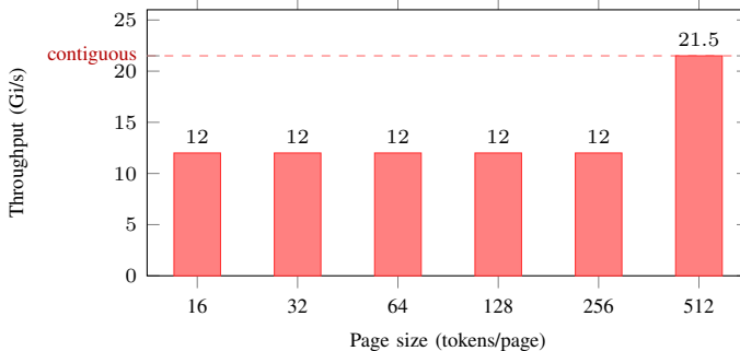
Fig. 6: Page size sweep ( N = 64 , \text{actual\_len}=512 , d = 128 ). Throughput is flat across all paged configurations. The \text{page}=512 bar reaches the contiguous baseline because each sequence fits in a single page with no indirection.
